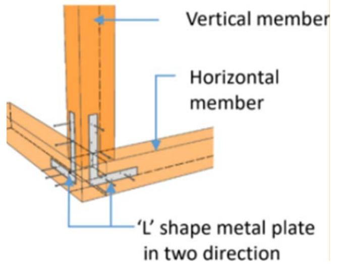
Figure 34: Detail at A: Connection at corners
