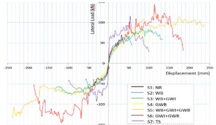
**Figure 18: Ultimate load and ultimate lateral displacement obtained from pushover tests conducted in stone masonry walls with various strengthening options**
