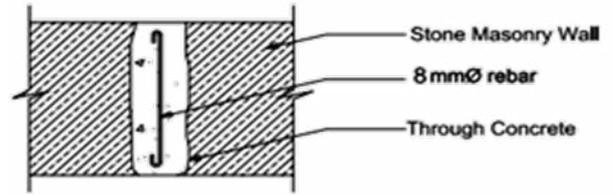
Figure 9: Through concrete in an existing SMM wall
